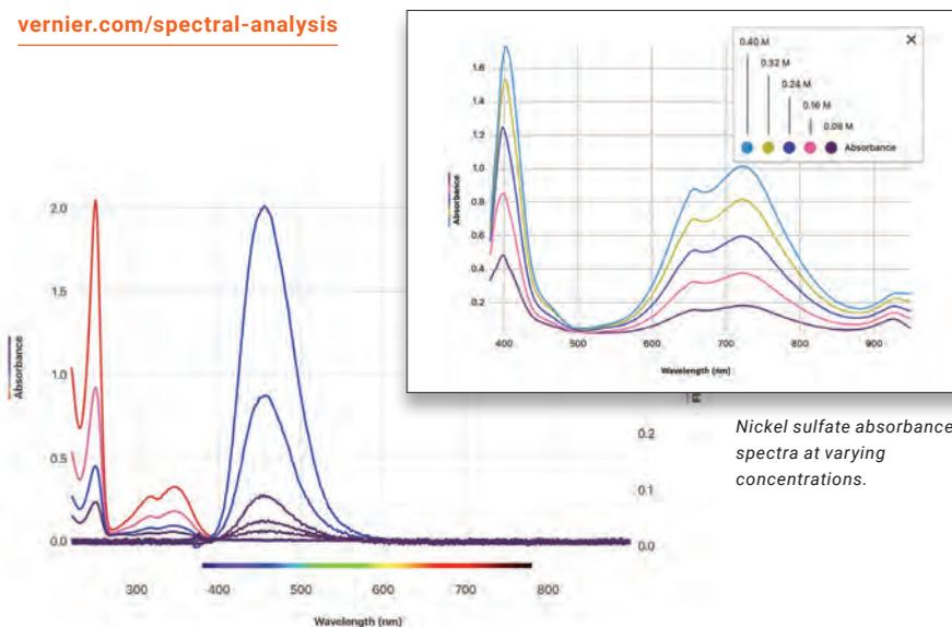
Nickel sulfate absorbance spectra at varying concentrations.
